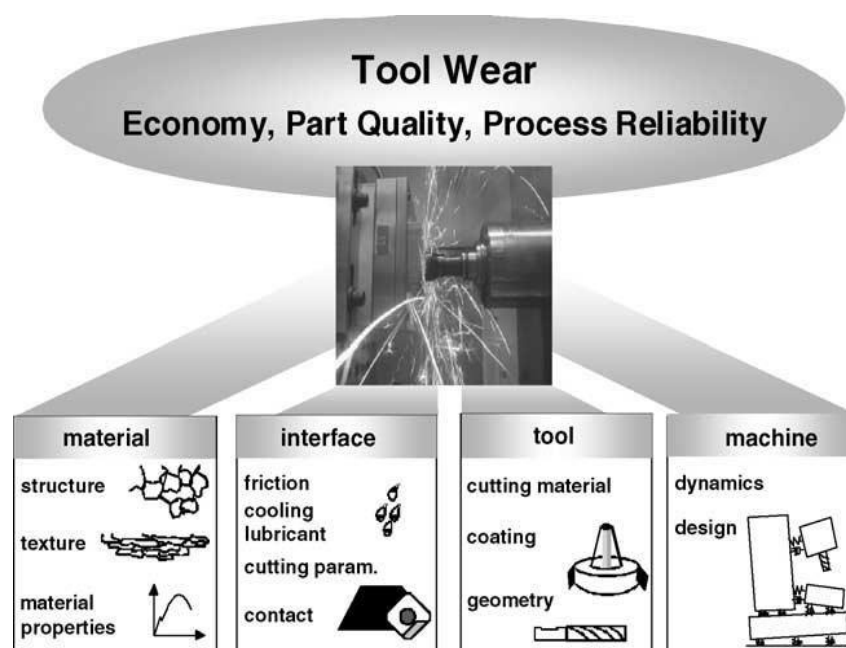
Fig.1.2: Four major functional elements influencing tool wear in machining processes. [Name of figures should be at bottom & bold]
